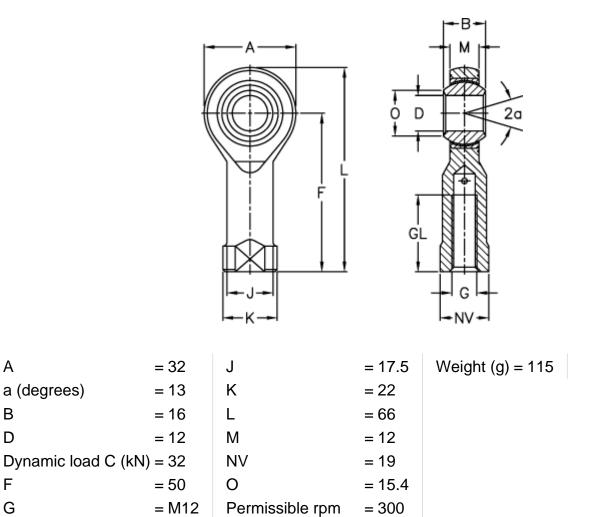
Static load C0 (kN) = 42
